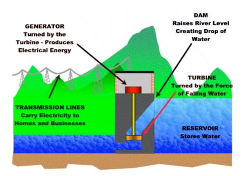
http://www.opg.com/ops/H how.asp schematic
